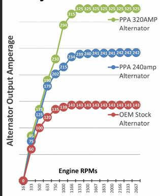
Our Pure Power alternators produce a minimum of 180 to 220 amps at idle. Best in its class!!!
